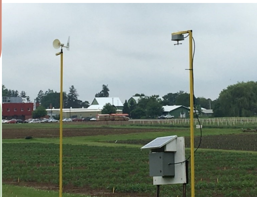
Figure 1. Spornado (left) and rotorod (right) spore traps setup at Ridgetown Campus, University of Guelph.
