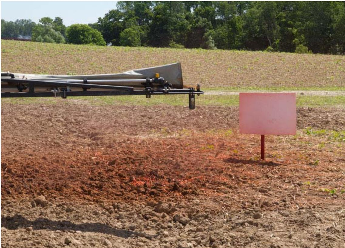
Demonstrating how fine droplets drift using food-grade red dye.
